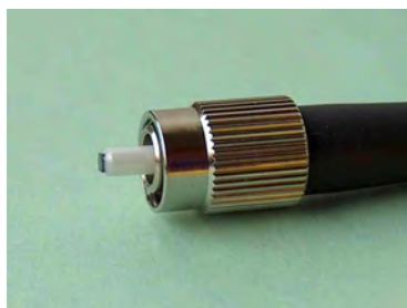
Figure 4.6.2: SAM chip on FC/PC connector end face
